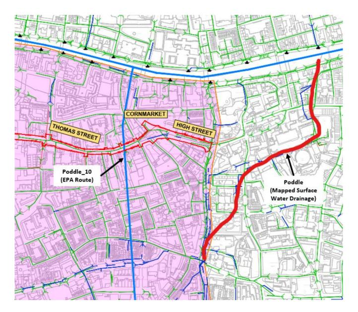
Image 13.2 Possible Route of Poddle\_010 (red line highlights surface water sewer)
